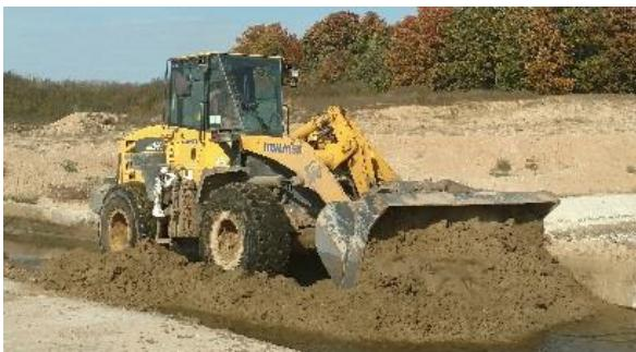
A concrete “sand lane” can be used to help separate sand from liquid manure, saving both the need to purchase more sand and wear and tear on pumping equipment.
