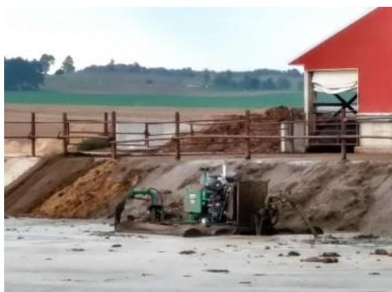
A John Deere “manure boat” is essentially a large air compressor outfitted with nozzles. It homogenizes the solids and the liquids so that they can be hauled and spread on crop fields where it can provide both nutrients and organic matter to the soil.
