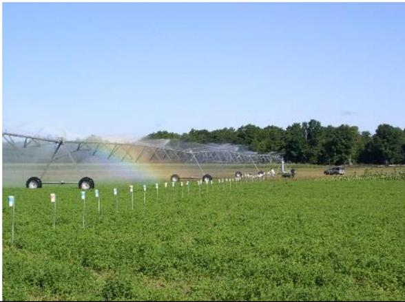
The “catch cups” placed along the length of this center pivot will help the farmer identify if there are any nozzles need repair, or if the rate and/or pressure needs to be increased or decreased to ensure the field is getting the water it needs.
